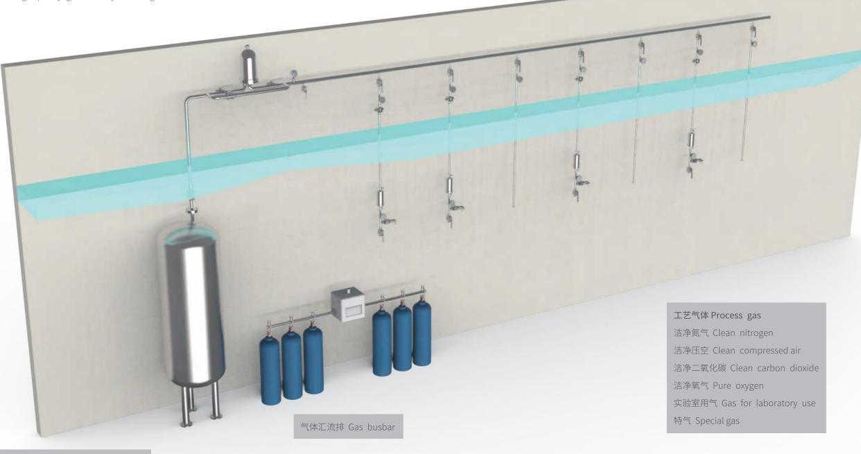
气体储罐可根据用户需求替换为分气缸或气体汇流排 Gas storage tank can be replaced with separate cylinders or gas busbars according to user requirement
